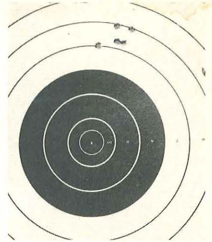
Group fired at 100 yd. after sighting in at 25 shows need for checking. The impact is 1 min. right, 1 1/2 min. high
