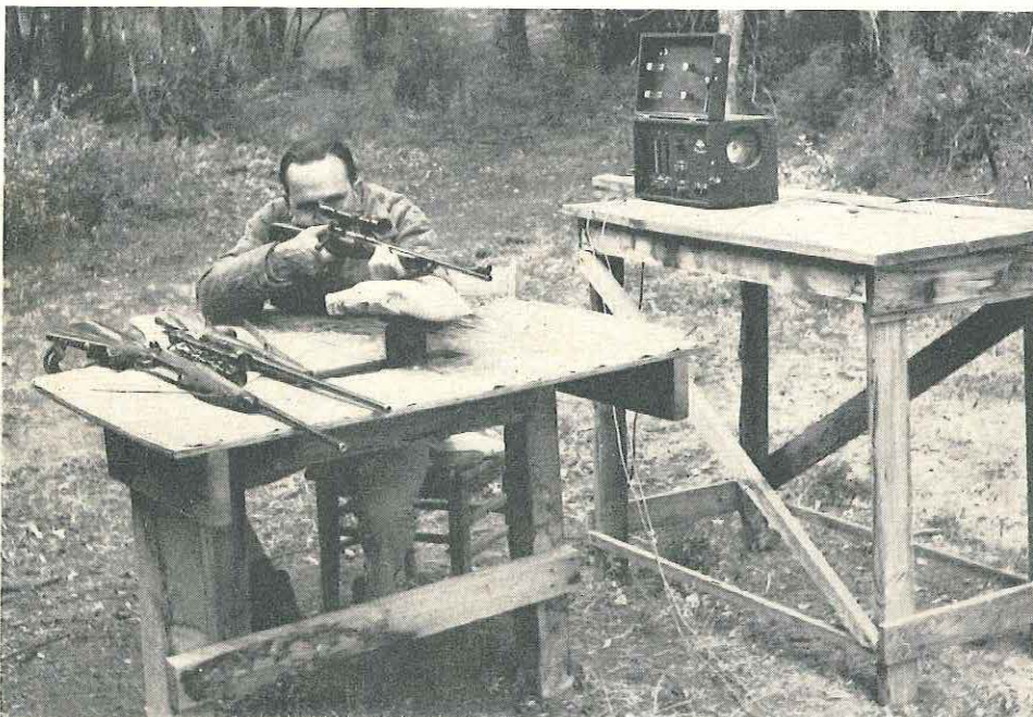
R. F. Chatfield-Taylor uses bench rest to sight in. Note chronograph on table at right
