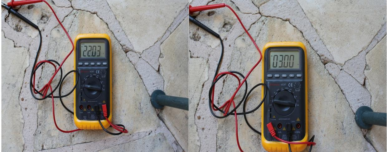
*The manufacturer claims you'll get up to 15 volts at 4 amps with this system. The panels were cranking out over 22 volts at 3 amps in the afternoon July sun. No sound, no gasoline. Just free flowing electrons ready to work for me.*
